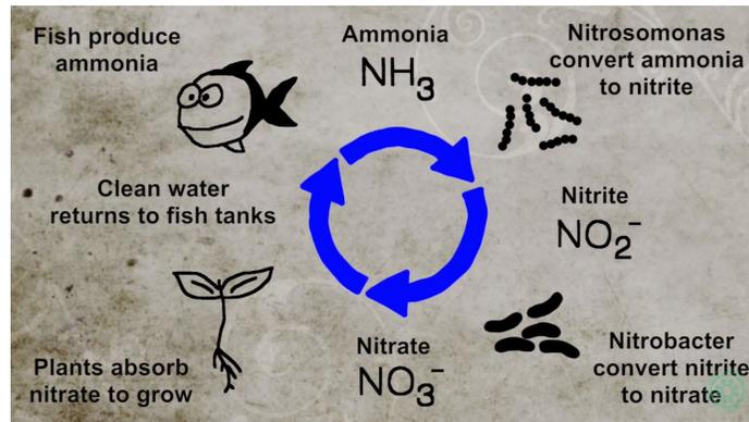
The process of nitrification, or the nitrogen cycle, is what converts the fish waste (ammonia) into plant fertilizer (nitrate) [20].
